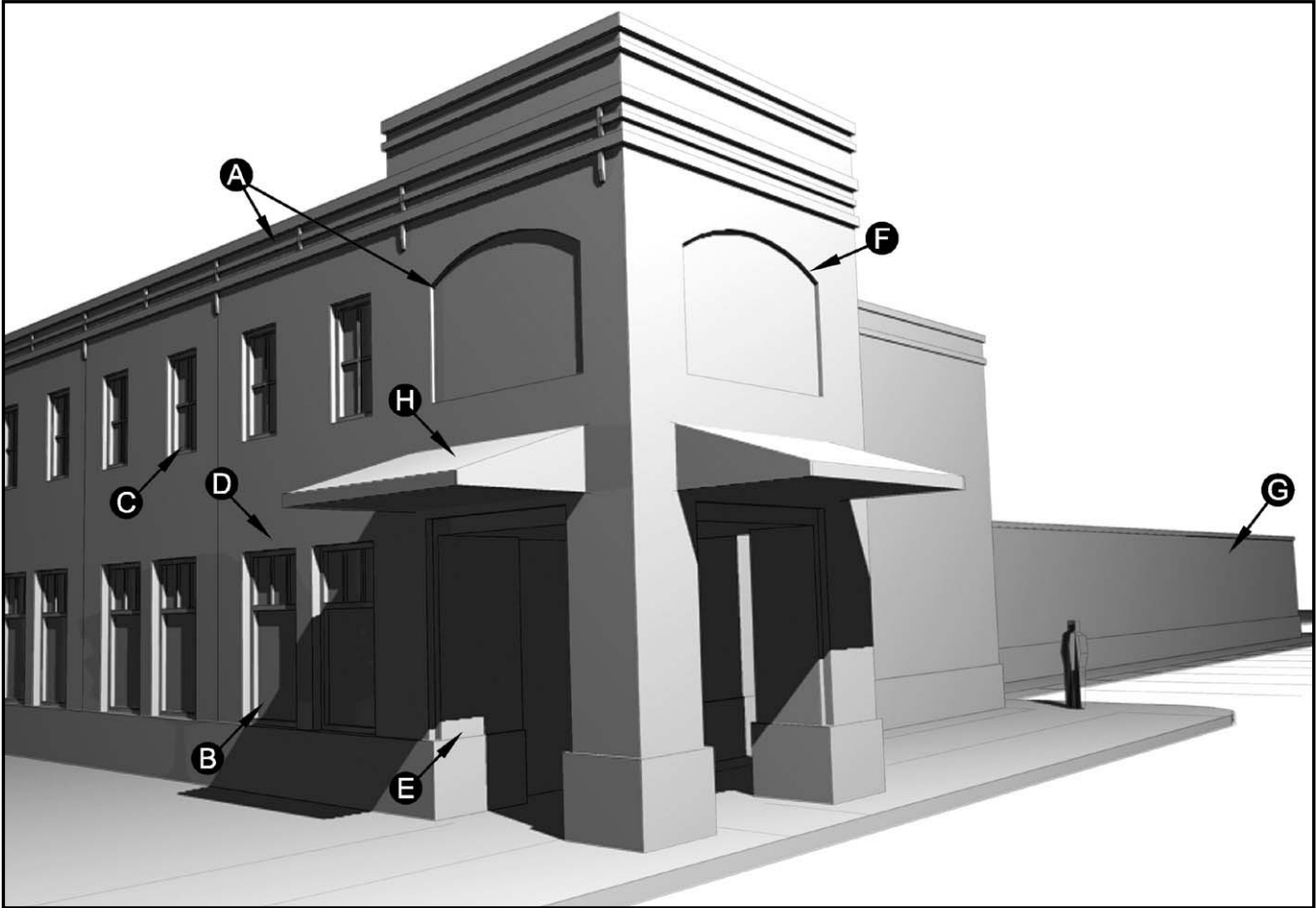
Figure 8: Fenestration Is A Measure Of The 3-Dimensional Depth Of A Façade Created By Fluctuations Or Openings In A Wall. Recesses such as archways or deep windows are two examples of fenestration. They help to give a façade a more 3-dimensional appearance by casting shadows and creating a visual contrast.
