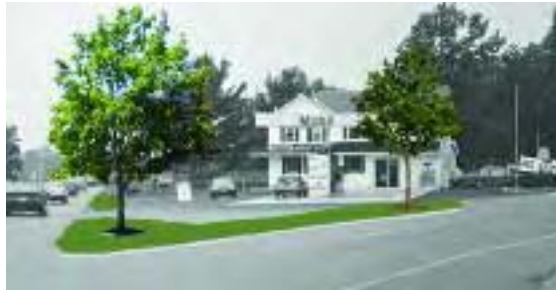
Figure 4.9: Limiting a Curb Cut to a Single Point. The wide, paved parking area and undefined access detracts from the scene at left and makes it a less attractive and less safe focal point for this intersection. An alternative shown at right provides landscaping for visual interest and to tie the site to the streetscape beyond.
