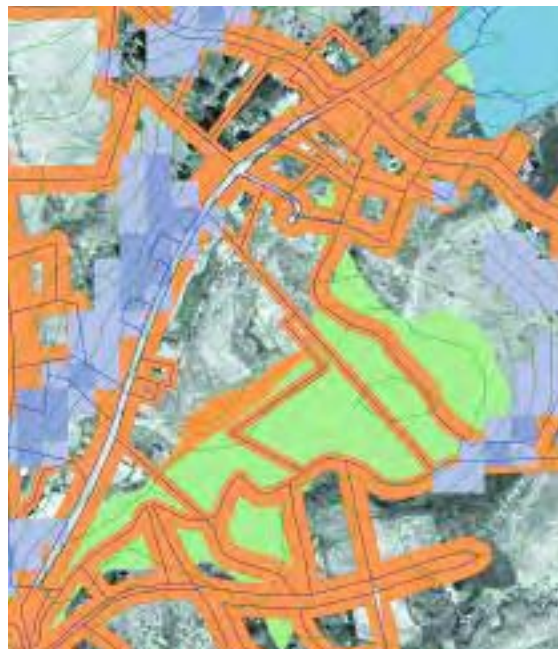
Figure 1.2: Landscape Inventory Map. A landscape inventory map contains the locations of site features that could restrict or encourage development. This one shows the base layer shown in Figure 1, with the locations of steep slopes (light and dark purple), floodplains (green), wetlands (blue), and no-build set-back areas (orange). When these "restricting" features are overlapped, the remaining land (gray) shows the areas most likely to be developed.
