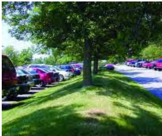
Figure 3.12: Breaking Parking Lots into Smaller Units through Landscaped Berms. Berms divide this parking lot into smaller units, reducing the visual impact of large expanses of paved or gravel surfaces. Plantings along the berms offer visual interest and have the added benefit of providing shade and reducing storm runoff.
